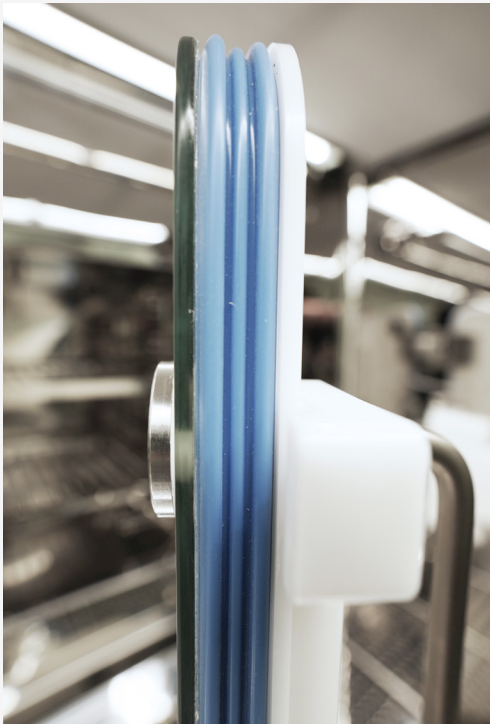
Incubator door with inflatable sealing.
